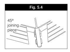
Insert the snap-in cover into the screw channel. Apply silicone sealant to the end caps and corner joining piece (if present), then insert them.
