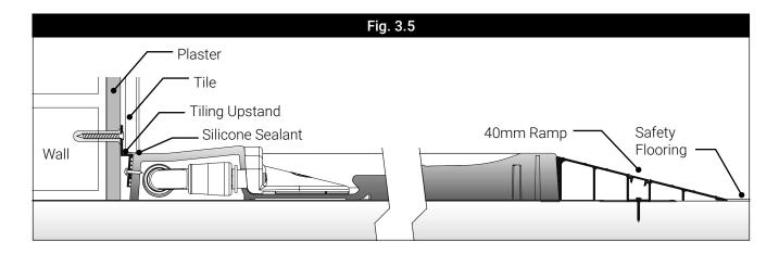
When using a 40 mm (11/2") ramp, install safety flooring up to and level with the ramp edge. If not installing a 40 mm (11/2") ramp, install safety flooring or tiles up to tray edge. See ramp installation.
